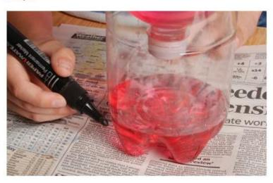
Pour the water into the top of the bottle and then start timing. Each time a minute passes, mark a line at the water level of the bottom bottle.
